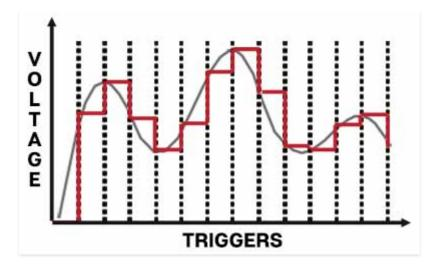
**Sample Source (Noise Gen) input and jack**- The noise generator is the default sample signal source. Because a noise source has all possible frequencies distributed in a random fashion, it makes an excellent source for "grabbing" completely random voltages. This signal can then be used to modulate oscillator pitch or filter frequency.
