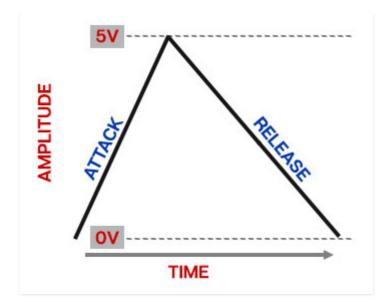
The AR envelope functions a little differently than the ADSR envelope. If the *Sustain* switch is on, it moves through the attack segment when a 5V gate is applied and remains at maximum as long as the gate voltage is present (equivalent to an ADSR envelope with its sustain control set to maximum). If the *Sustain* switch is off, it moves through the release segment regardless of whether the 5V gate voltage is present.
