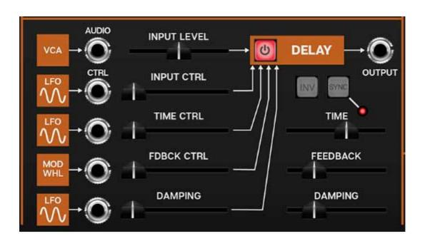
**On/Off**- The red button in the orange box enables and disables the delay effect.
