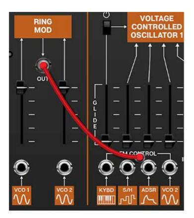
Patching A Cable- Simply click on a jack, drag the cable to the desired destination jack and release the mouse button. Cables can be
