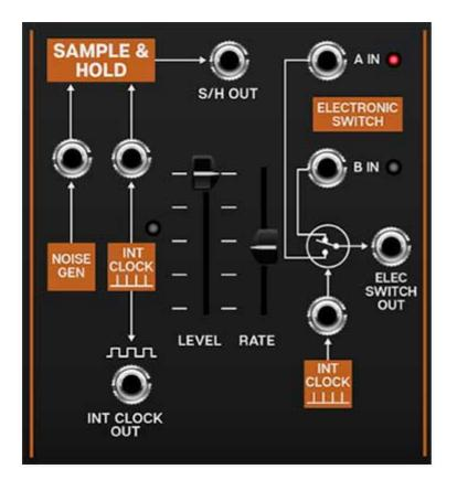
The sample and hold section repeatedly "samples" a varying input signal voltage, and outputs the "snapshot" voltage (i.e. a constant voltage) until it is triggered to sample again. Note that when we say "sample," we're referring to a simple incoming voltage - this isn't an audio sampler that you can sample and playback beats with. (Though this is the basic principle of how digital audio samplers operate).
