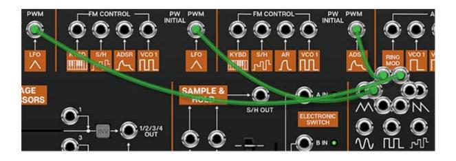
In the image above, we've routed three cables from the LFO ramp wave output to the PWM inputs of each oscillator. Single-clicking on any CA2600 input or output jack reveals a six-way multiple jack (aka, a "mult"), which is super convenient for routing or mixing multiple sources. The mult stays visible while routing or if the mouse is hovering on it, and is hidden when a cable is routed.
