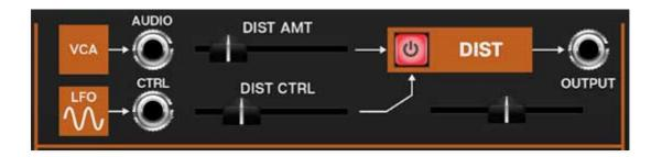
**On/Off**- The red button in the orange box enables and disables the distortion effect.
